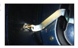
Remove the right rear trunk bolt and install the provided metal grounding bracket at this point and to the lower mounting hole of the antenna base.
